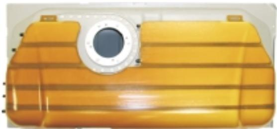
high-speed, rear-end impacts have cost police officers their lives from otherwise survivable collisions. A custom version of the FIRE Panel was specifically designed to perfectly fit the contours of the police car's fuel tank, thus adding a strong layer of fire protection for the officers.
