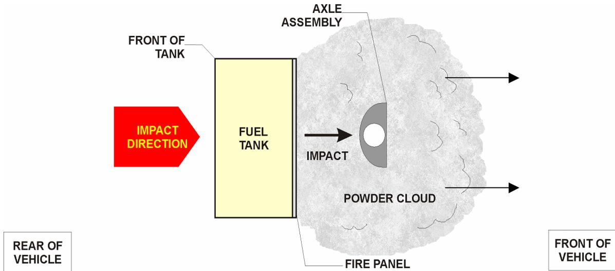
**Fig. 2 - Normal Impact Schematic (Side View)**
