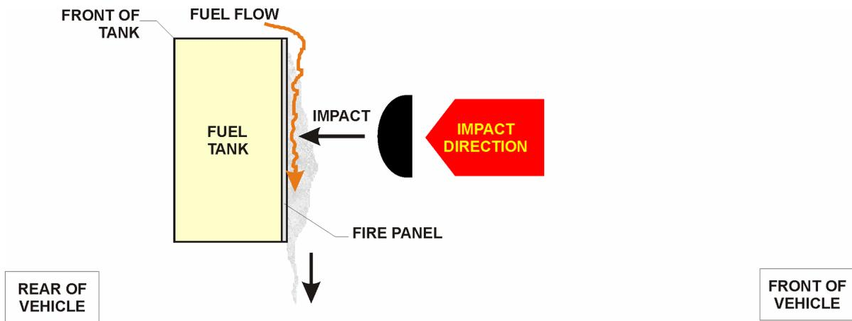
Fig. 2 - Ford Test Schematic (Side View)
