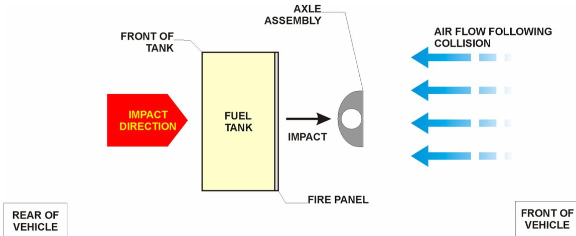
Fig. 1 - Normal Impact Schematic (Side View)
